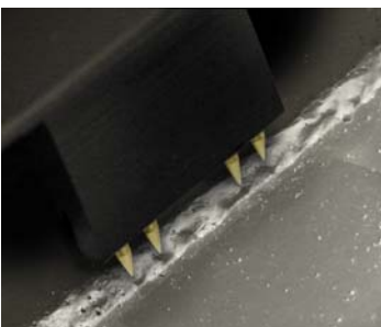
Close-up of the DRM-4012 probe's contacts
