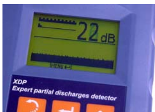
The XDP display while in use: it indicates the intensity level of the signal and its wave form.
