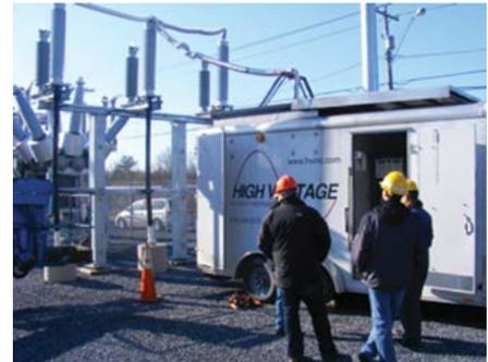
200 kV VLF van in service, high voltage out thru top.
