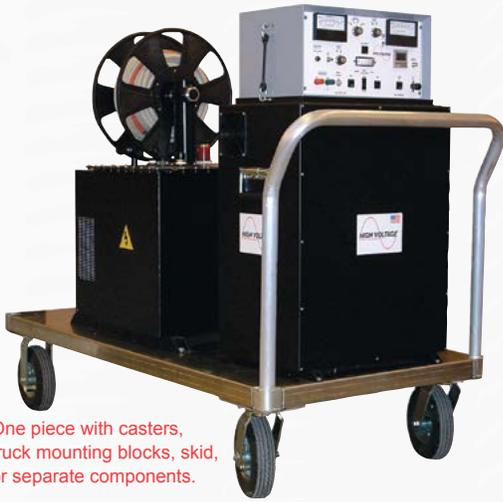
One piece with casters, truck mounting blocks, skid, or separate components.
