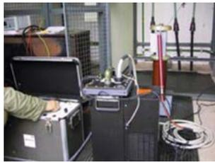
**$\mu$ F Rating:** VLF hipots are rated by the capacitance of the loads they can test. To select the right model, either the load capacitance must be known or the cable length if the  $\mu$ F/km,  $\mu$ F/ft, etc. is known.
