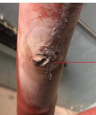
**Real case scenario:** Partial discharge detected on a cable termination by the PD Annunciator™ system with SonoTEV™ and HFCT-HD™ sensors.
