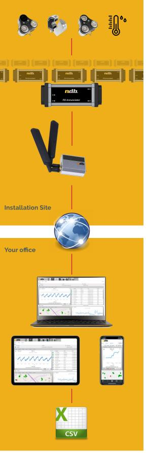
Data Export: PDA-Cloud™ provides easy data exportation to flexible .csv file. Raw data is then easily imported to your company's database for trending evolution of partial discharge.
